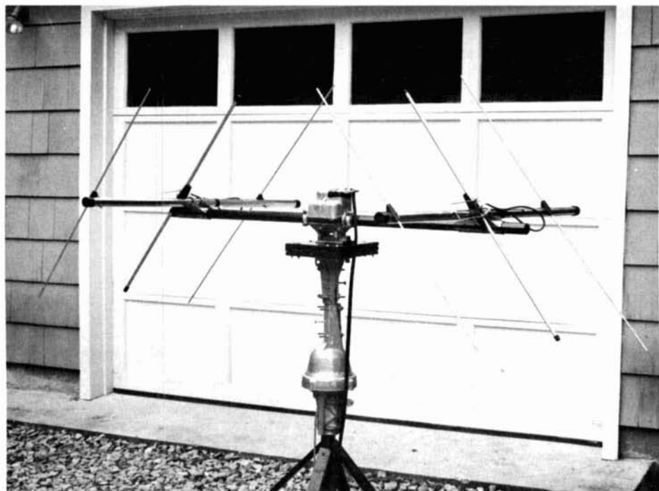
fig. 5. Az-el mount assembled using two 3-element 144 MHz Yagis at 90^\circ to each other for circular polarization. Cross boom extends through U-100 rotor. Feed line and phasing harness not shown.
